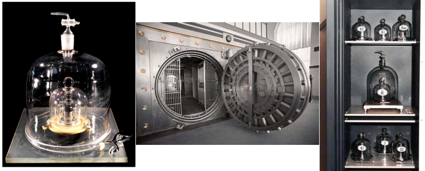
International Prototype Kilogram (IPK) – definition of kilogram since 1889. Mass standards are traceable to the IPK, comparison at BIPM.
